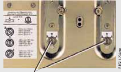
Adjusters (on the rear side of the device) to set the site altitude
